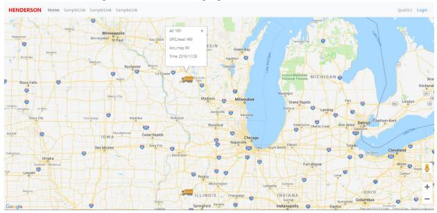
• For admin/user view: Admin managers can access all information in our design, road conditions, truck's path, truck information (e.g. altitude, GPS, acceleration, conveyor speed, spinner speed). The top-right corner of figure below shows that the it has logged in as user, and we have nothing for road conditions to show on our map now.
